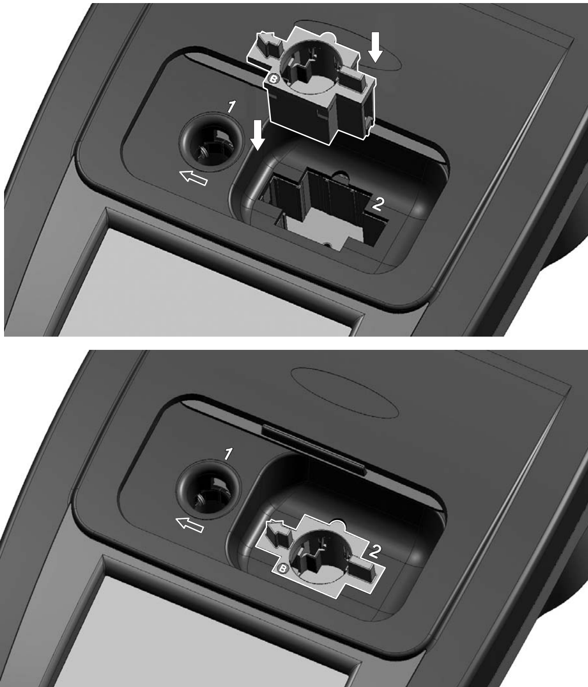
Figure 4 Installation of a cuvette/sample cell adapter
