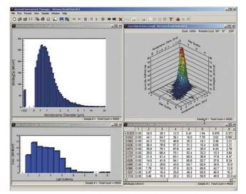
Aerodynamic diameter and events displayed simultaneously
