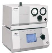
APS configured with optional Aerosol Diluter (Model 3302A) for conditioning high-concentration aerosols.
