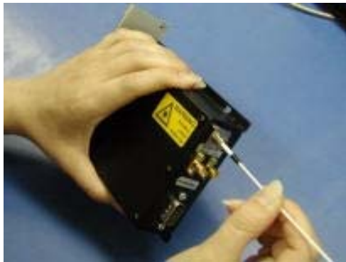
Figure 22 Cleaning the Optical Port [2]
