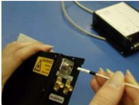
Figure 21 Cleaning the Optical Port
