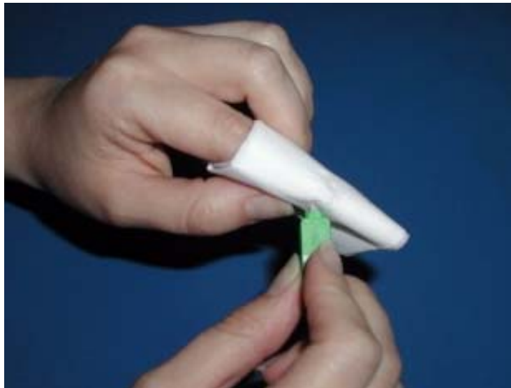
Figure 19 Wiping the connector with a Kim wiper
