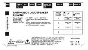
Audio source is connected to the audio IN socket with a 3,5mm stereo jack. Audio source may be any source with output level from 50 mV to 2 V. In case of connected audio player the normal audio cable with 3,5mm stereo jacks provided by the user should not be longer than 3 meters. This is for the installation to meet the strict EMC regula-
