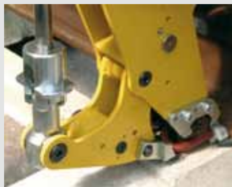
Extraction and insertion of Pandrol "fast clips".
