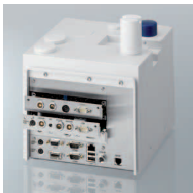
Additional sensor boards are easily plugged in.
