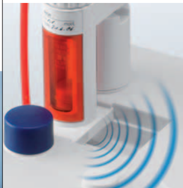
The burette data is automatically read by the RFID sensor.
