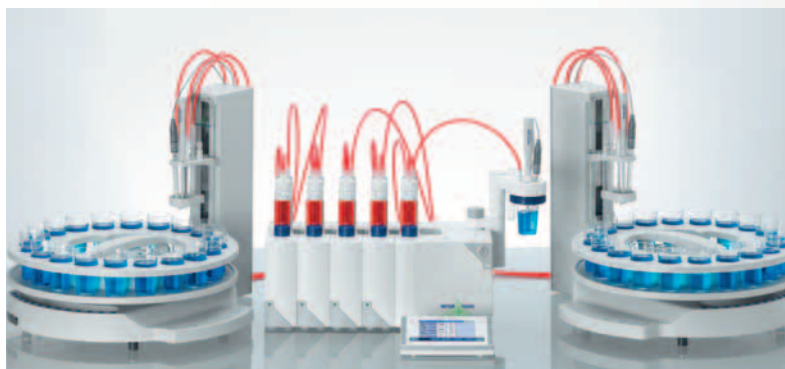
Up to two Rondo can operate with a T90 in parallel – even without PC software.
