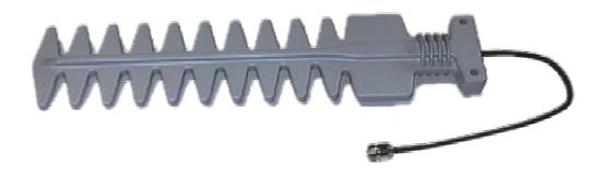
This antenna covers the 1.4 - 1.5 GHz WorldSpace frequency range. This is a yagi antenna inside a moulded plastic enclosure. The antenna is for receiving digital audio broadcast (DAB) and WorldSpace Satellite radio. The antenna has been designed to be waterproof and is easy to install. It is supplied with a mounting bracket that allows it to be fixed to pipes. Elevation for 0-90 degrees is provided for.
