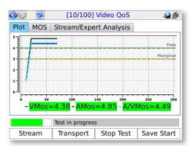
display of IP Video results. Tech-X Flex gives a Video MOS score (VMOS) which rates the customer's QoE with a number between 1 and 5. The closer to 5, the better the experience. This provides a quick and easy method for the technician to evaluate the customer's service. However, should a more detailed analysis be required, Tech-X Flex also provides additional measurements such as jitter, I/B/F frame counts, loss and more.
