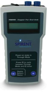
For all copper testing that specifically indicates RU support, the Tech-X Flex WB Copper module automatically controls the RU through DTMF tones and no manual intervention is required.
