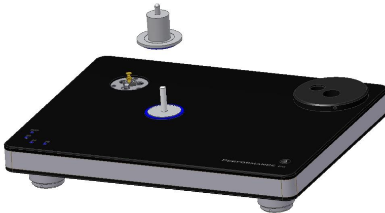
Pic. 5: Fitting the bearing upper part
