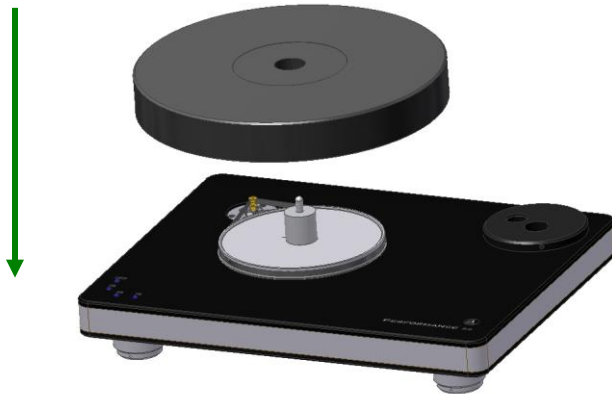
Pic. 7: Setting the platter onto the bearing
