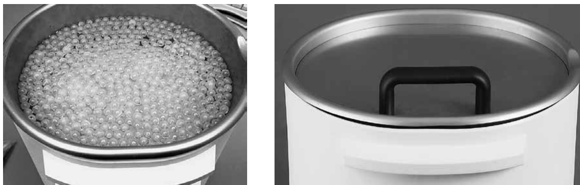
Fig. 5.2: Floating balls in the heating bath medium and cover for heating bath
