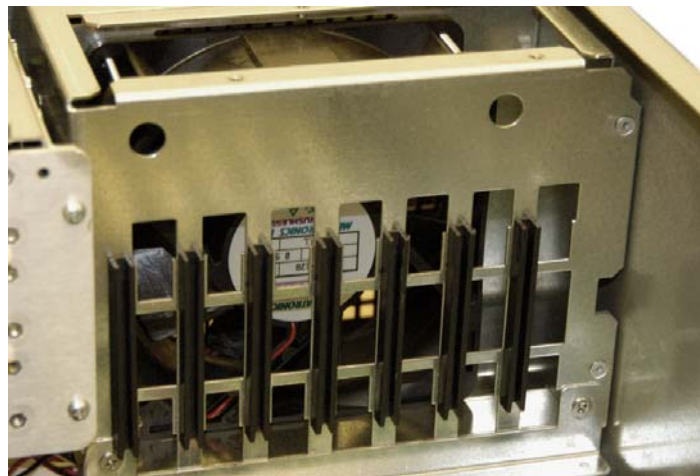
Figure 5-18: Access Holes To Fan Retaining Screws
