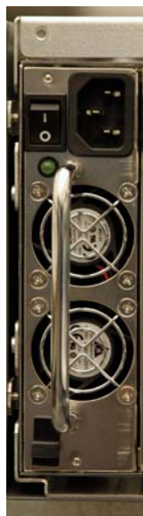
Figure 5-14: Power Supply ready to be removed.
