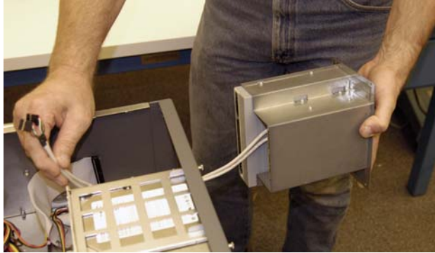
Figure 5-22: Removal of DVD/CD and Floppy Drive
