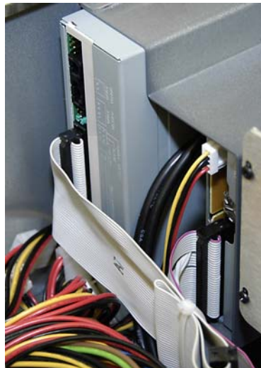
Figure 5-21: Motherboard ribbon and power cables connected to DVD/CD and Floppy Drive
