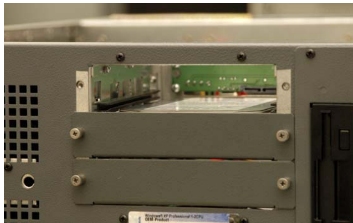
Figure 5-12: View of empty hard drive bay
