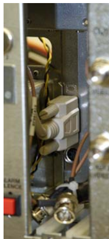
Figure 5-8: Monitor cable connected to SVGA card.
