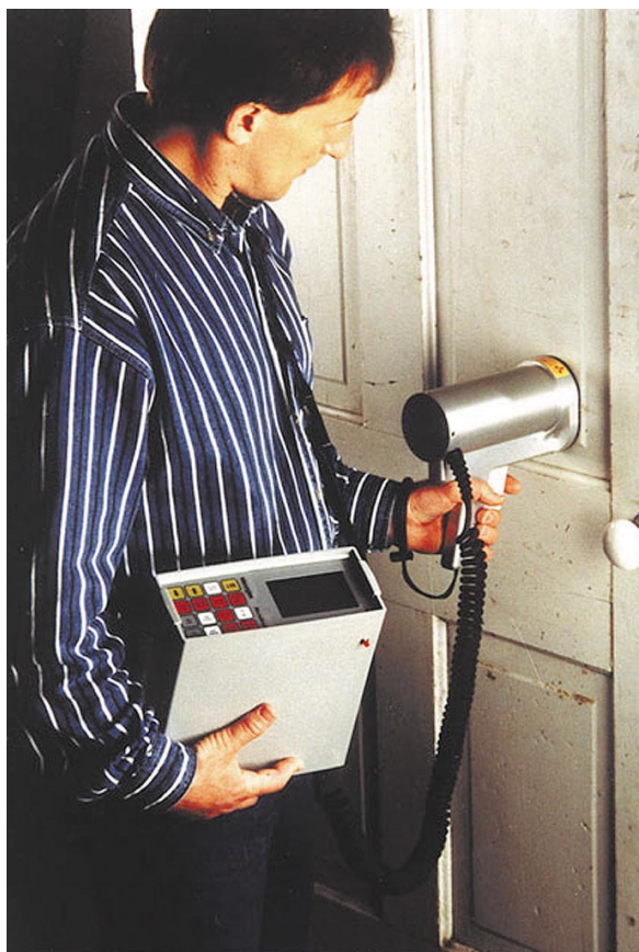
Fast measurement of lead concentration in a door with Microlead I
