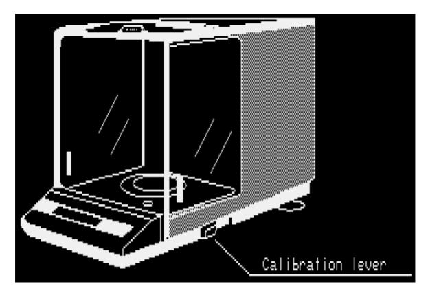
Once having moved the calibration lever to the rear, the display will change to:
