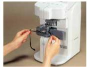
**Automatic judgment for a progressive lens**You can automatically check whether the lens is a progressive lens or not. FAR POINT and NEAR POINT can be easily measured by directions and a graph display of color LCD screen.
