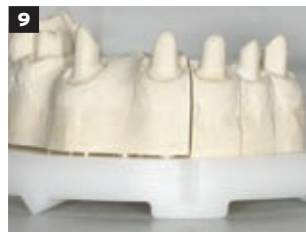
9 The linear expansion tension is released; the segments drop back flush with base plate. The saw cut "eliminates" the expansion
