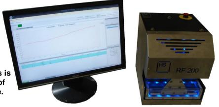
The measuring object is placed in a heated water bath. The included software starts the measurement. An Init-program considers the force of the water. The start value is determined using a force threshold value. The further process steps in the program are then processed. It is thus possible to cover a wide process window with just one program.
