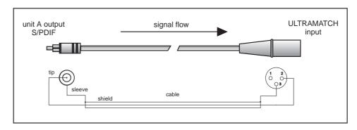
Fig. 3.6: Adapter Wiring for RCA Output to ULTRAMATCH's XLR Input
