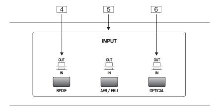
Fig. 4.2: Controls of the Input Section
