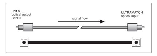
Fig. 3.3: Optical Connection via TOSLINK (SPDIF) to the ULTRAMATCH
