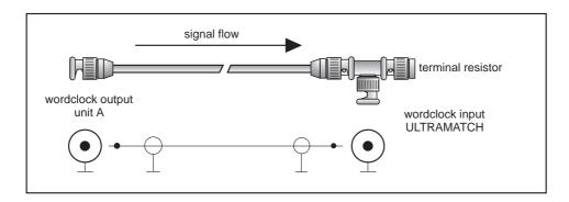
Fig. 3.4: Termination Connection of the Wordclock Input of the ULTRAMATCH
