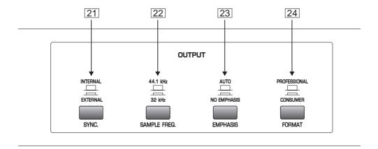
Fig. 4.4: Controls of the Output Section
