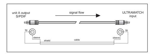
Fig. 3.2: Unbalanced Connections (SPDIF) to the ULTRAMATCH
