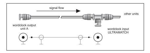
Fig. 3.5: Passing through connection of the Wordclock Input of the ULTRAMATCH
