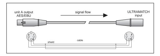
Fig. 3.1: Balanced Connections (AES / EBU) to the ULTRAMATCH
