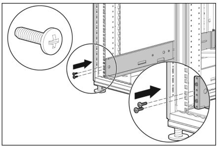
4. Insert screws through the rack into the mounting rail and the rear of each mounting bracket. Do not tighten.
