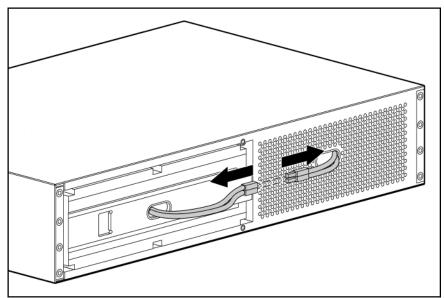
4. Remove the battery bracket.
