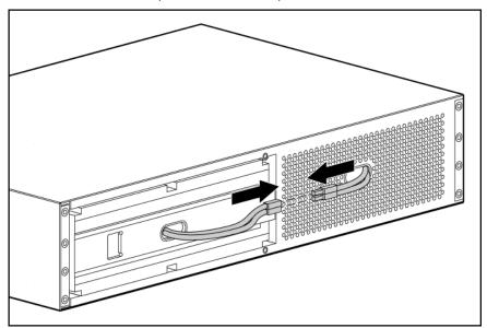
**NOTE:** A small amount of arcing may occur when connecting the batteries. This is normal and does not damage the unit or present any safety concern.
