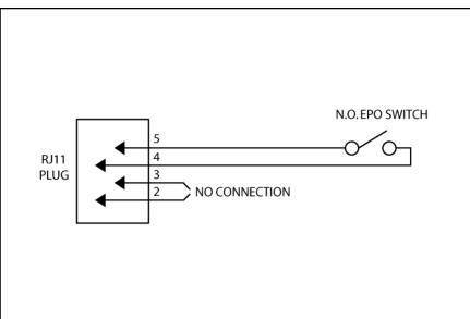
When the switch is enabled:
