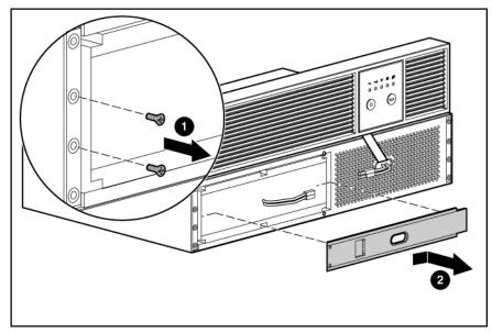
5. Remove the UPS battery modules.
