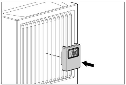
3. From inside the bezel, gently push out the LED/Control panel, rotate it 90 degrees, and then replace it in the bezel.
