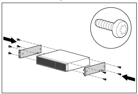
1. Attach the 2U side-mounting brackets to the unit.
