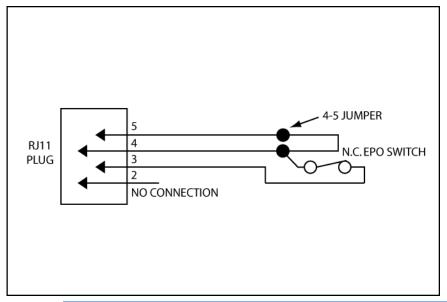
**NOTE:** If the UPS was operating on battery power when the remote switch was closed, no power is available to the load devices until utility power is restored and the UPS has been manually powered up.
